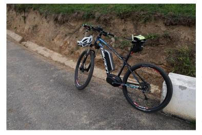
Frame: 27.5" 27225, Alloy 6061 Fork: Rockshox XC30 Air 120mm Brakes: Shimano M447 Hydraulic, Mineral Oil, discs Shimano 180mm front 160mm rear Whels: Rims WTB Disk i19 27.5, hub X7; tires Continental X-King 2.2 Trasmions: rear X9 10vit, maneta X7 10vit Handlebar: Devron 600mm, Rise 0; Pipe Truvativ, saddle: WTB Silverado Engine/Display/Sensor: BAFANG, 36/43/48V; 250-350W, 90-120 RPM, Cuplu 80N.m, Efficency: ≥ 80%, weight:3,8kg, Noise: <55dB
