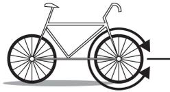
To get the accurate result, the wheel size should be correct. Mark the symbol on the tire and ride one circle. Then measure the length between two points that will be the circumference.
