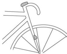
Check the position of the front fork to find the suitable point to attach the speed sensor. The distance between CY-200W & the speed sensor would be in 600mm.
