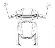
1. The rear hydraulic brake is operated by the left brake lever. Pressing it will operate the rear drum brake.
