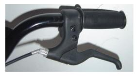
2. Insert the brake cable wire into the slot in the front of the brake lever and then remove your hand. The brake cable cap will automatically spring back into the slot on the front of the brake lever assemble.
