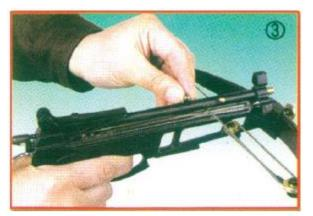
Pulling: Pull the string hook with force until it is secured in the pin. (If the alternative firing button is pulled out, the lock will release, and the ball will fit into the groove). Pic. 4 and 5.
