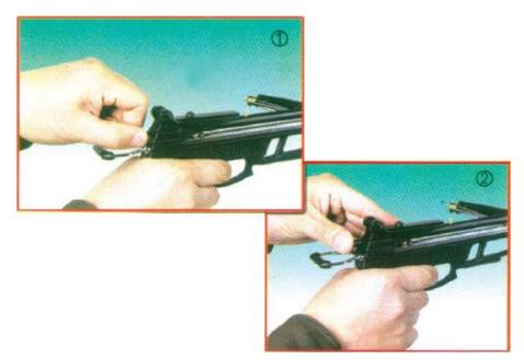
Loading: Push the loading button forward and jam into the right notch so that it does not return. After loading, return the loading button to its original position. Pic. 3.
