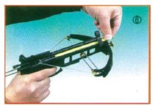
Placing the harpoon: If you want to shoot the harpoon, the hook must be placed downwards. Pic. 7.
